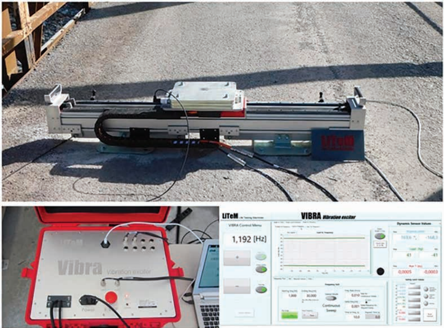
Fig. 6 | Vibrodina lineare VIBRA 9001, controller e software – Litem - life testing machine
